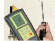
Open the air band on the burner to reduce your CO<sub>2</sub> lecture by 1.5% with a two pipes installation. On a one pipe installation reduce your CO<sub>2</sub> by 1%.
